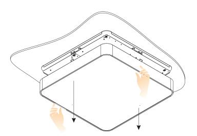
Pull down the luminaire's base in order to expose the mounting springs.
